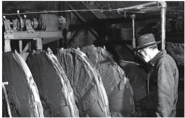
Disc filters were the last stage of concentrate production, drying it before shipment to smelter
